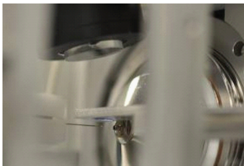
Figure 1. Backside illumination configuration with sample target between the laser focusing lens and the electrospray.
