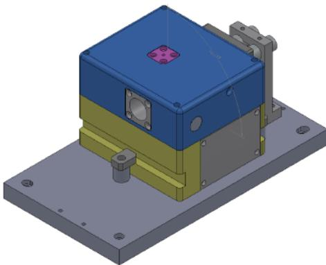
System includes an alignment kit for precise positioning of OPO module in pump laser beam path.
