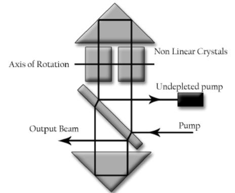
Ring-Cavity™ design cancels walk-off, eliminates beam steering and produces highly stable and efficient output.
