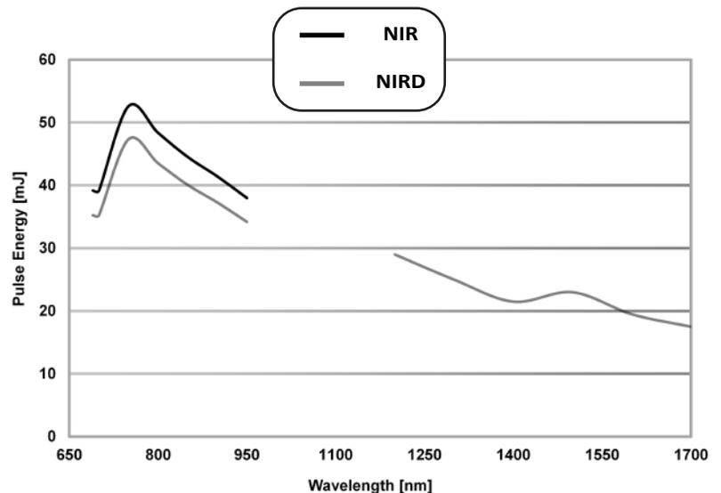
Typical performance when pumped with 140 mJ of 532 nm. Actual results may vary depending on pump laser.
