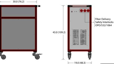
OPO Laser Head OPO Control Electronics Pump Laser Power Supply 210 lbs (95 kg)
