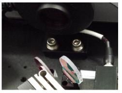
Built in Energymeter<sup>™</sup> monitors OPO pulse energy in real-time and provides feed-back for harmonics auto-optimization and logs pulse energy for data normalization.
