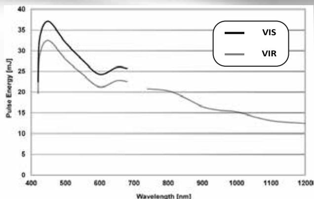
Typical performance when pumped with 90 mJ of 355 nm. Actual results may vary depending on pump laser.
