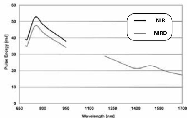
Typical performance when pumped with 140 mJ of 532 nm. Actual results may vary depending on pump laser.
